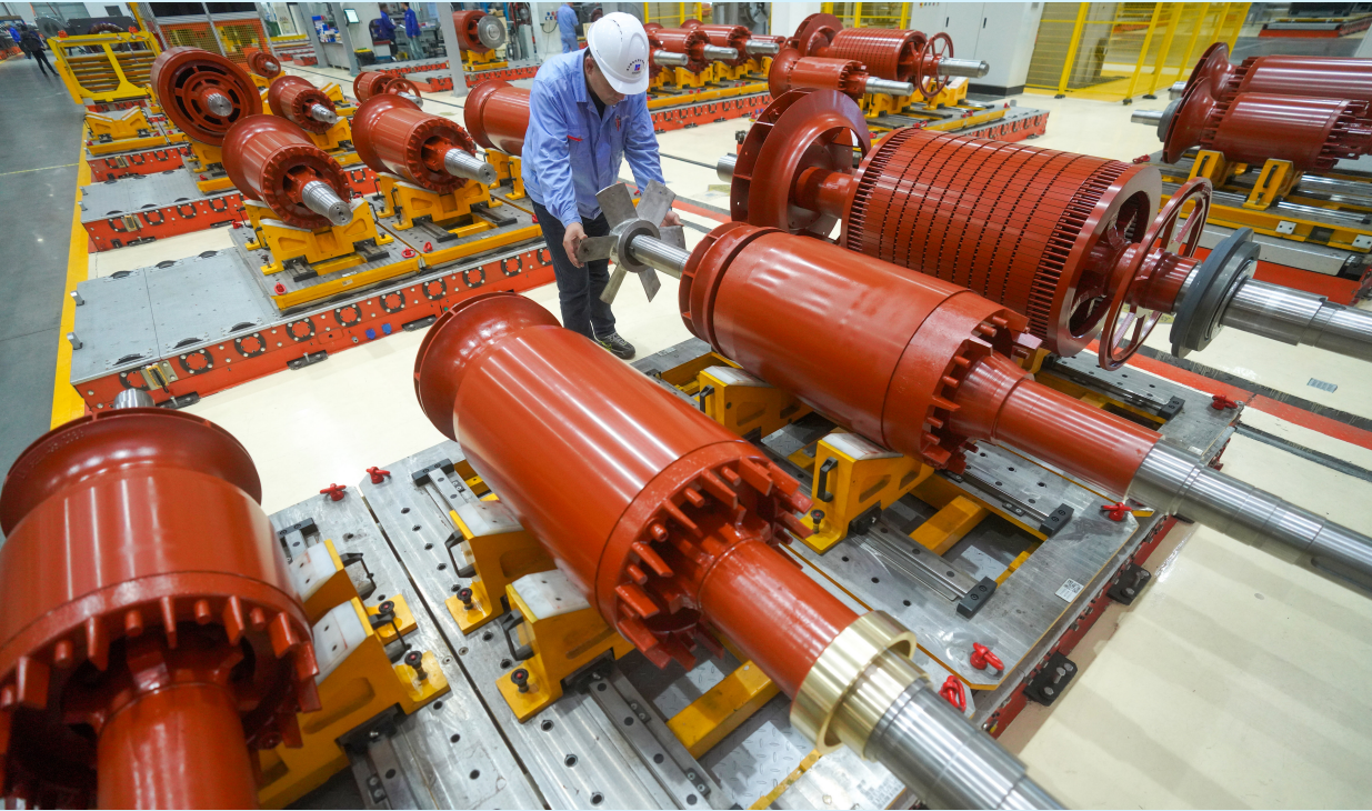
The quality inspector is checking the apparent mass of the fan inside the rotor
