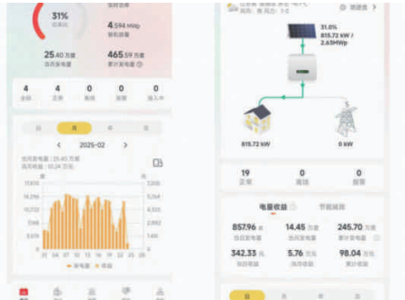
Handler’s Online Power Monitoring Platform – PV Generation Monitoring
