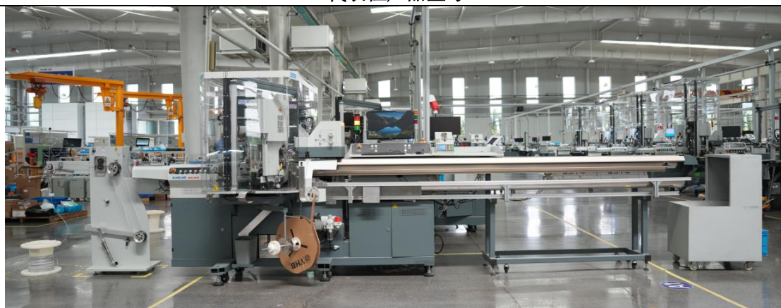
HBQ-804E 型全自动下线压接机 (长宽高: 3.8m*1.5m*1.9m)
