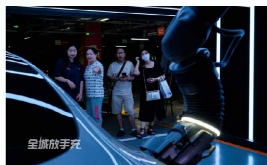
The "flexible arm + embodied AI" solution resolves the industry pain point of cross-vehicle charging adaptation 「柔韌臂+具身AI」破解跨車型適配難題
