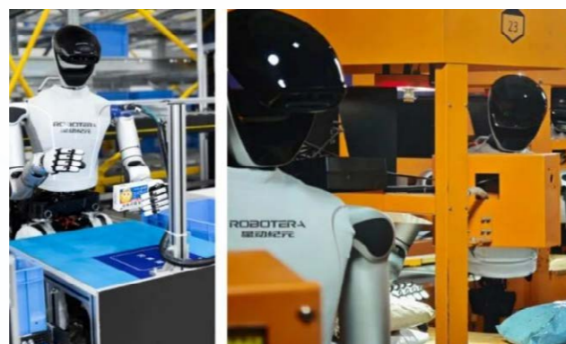
Robotera humanoid robots perform pharmaceutical sorting and logistics parcel feeding operations in factories
