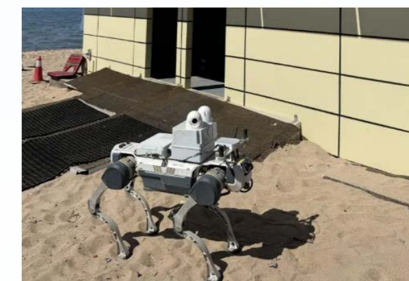
Deep Robotics' Jueying X30 robot dog for fully automatic outdoor inspection 雲深處絕影 X30 機器狗全自動戶外巡檢
