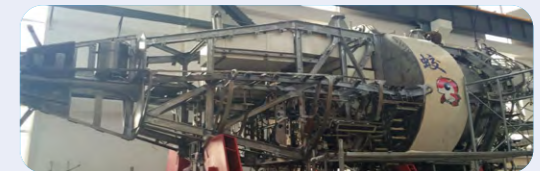
“蛟龙”号现场检修
