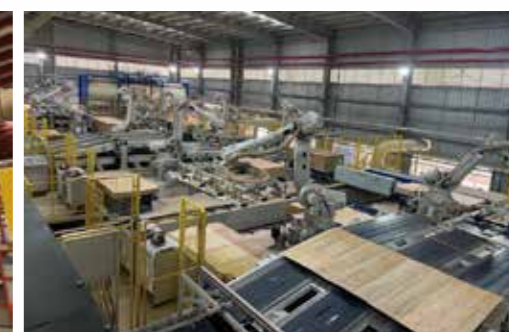
Plywood production line: automatic robotic veneer layout
