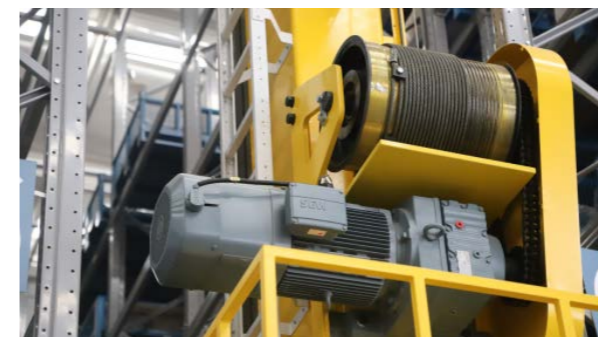
Stacker crane kinetic energy recovery system
