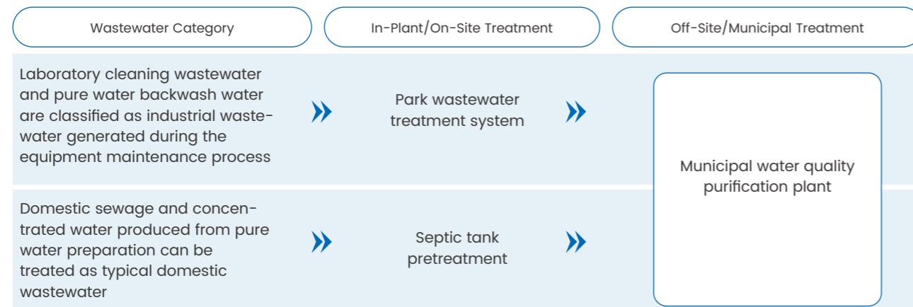
The Company's Wastewater Treatment Process
