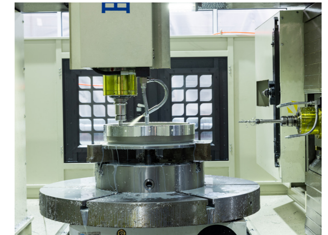
VMC Series Vertical-Horizontal Combined Machining Center
