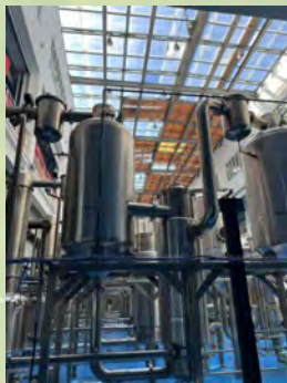
The extraction workshops use a natural daylighting design 提取車間自然採光
