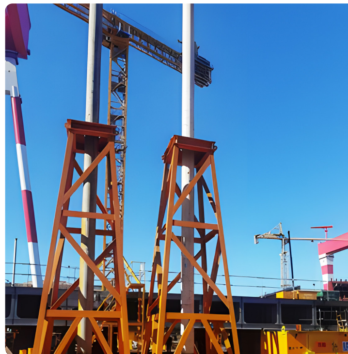
Stabilizer frame adopting spiral support structure
