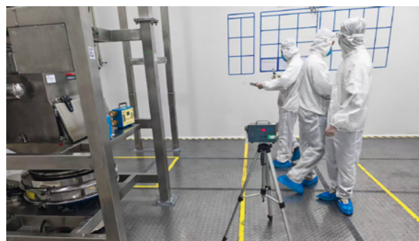
Changhong Newenergy conducts noise monitoring
