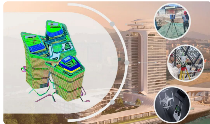
Reverse modelling of the engineering structure using 3D LiDAR scanning measurements 對工程結構採用三維激光雷達掃描測量進行逆向建模
