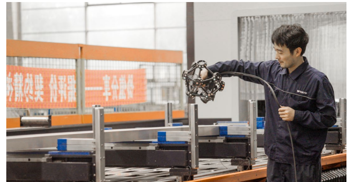
3D scan modelling of doubly curved engineering machining objects 雙曲工程加工對象3D掃描建模
