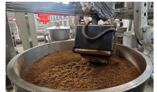
Gujing Distillery uses intelligent robotic steam probing for loading steaming fermented materials.
