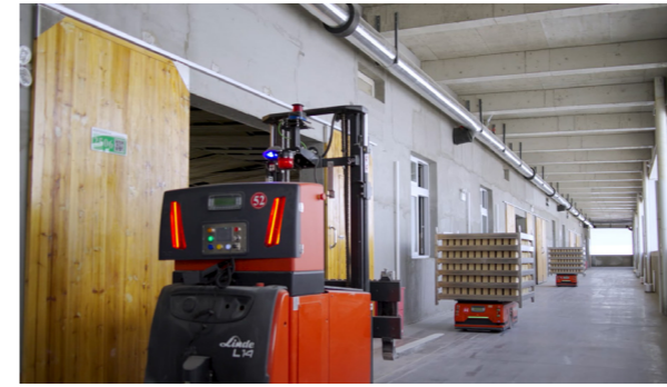
AGV Unmanned Material-transporting Vehicle, AGV Qu-turning Forklift
