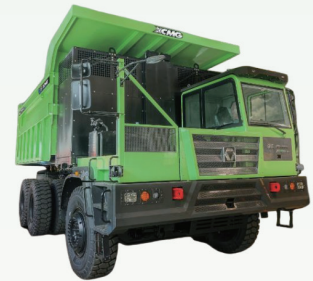
XGE150 Pro— 90-Ton Class Electric Mining Wide-Body Truck With Full Hydro-Pneumatic Suspension
