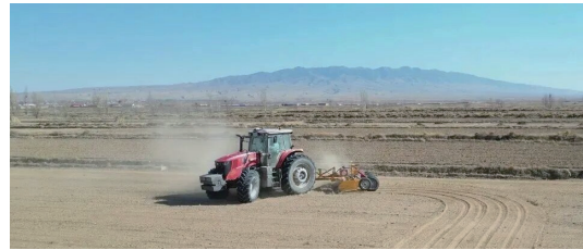
XCMG XT2204-6DK tractor pulls a land leveler to perform land leveling for corn sowing in Ningxia Plain
