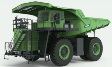
XDE130E —120-Ton Class MW-Level Ultra-Fast Charging Pure Electric Dual-Axle Rigid Mining Truck
