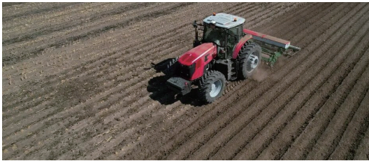
XCMG XT2204-6DK tractor pulls a rotary tillage & ridging integrated machine for fine soil preparation operation in Gongzhuling, Jilin
