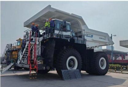
XDE150E—140-Ton Class MW-Level Ultra-Fast Charging Pure Electric Dual-Axle Rigid Mining Truck
