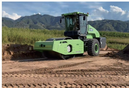
XS265EP—The World's First Electric Roller With Dual-Motor Drive
