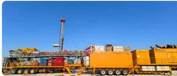
Oman (Middle East), "New Generation Electric Workover Rig with Energy Storage and Saving System" project in Ghaba area of Dhahira Governorate, contributing to green transformation of traditional oil fields
