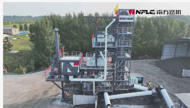
RAP Fine Stripping and Screening Aggregate Recycling Plant
