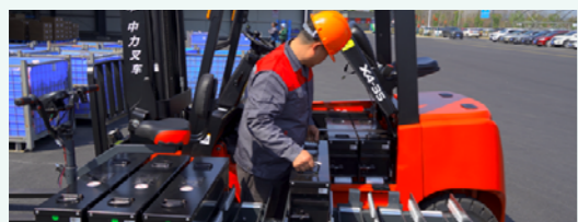
EP Forklift Battery Swapping Station (top) Modular Lithium-Ion Battery Pack Forklift (bottom)
