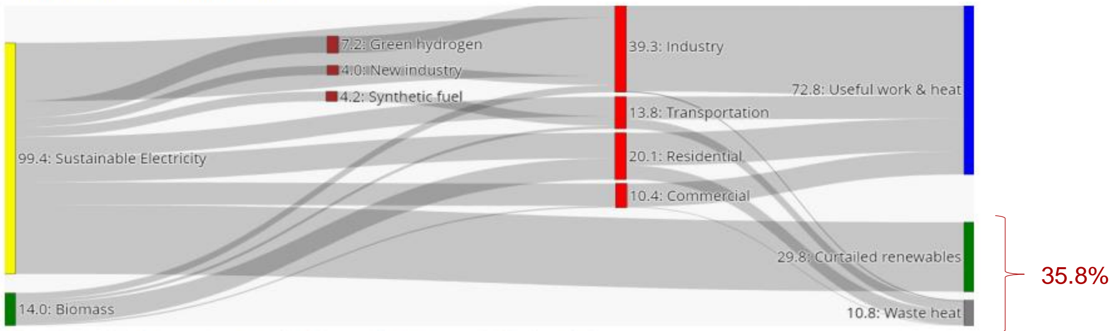
Figure 15: Sustainable Energy Economy, Global Energy Flow by Sector, IEA &amp; Tesla analysis
