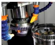
**原理：**用插齿刀按展成法或成形法加工齿轮
