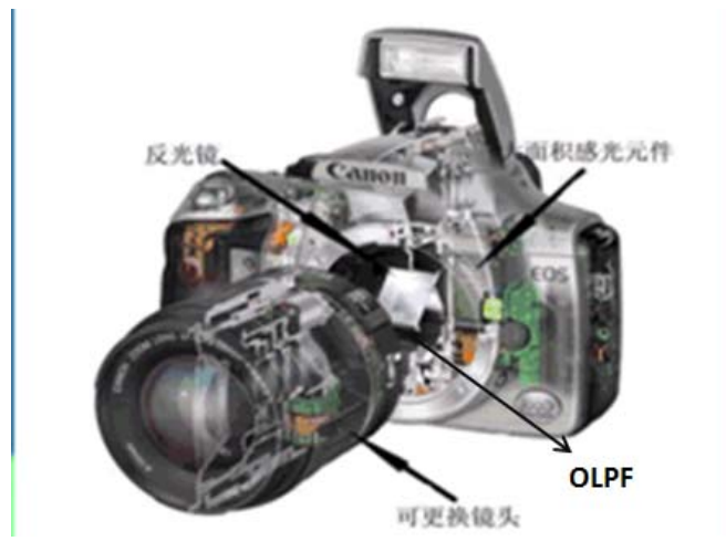
Exhibit 4: OLPF is used in front of DSC CMOS to eliminate color Moire fringes OLPF in DSLR
