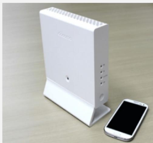
Fig. 1: NTT DoCoMo's dual-mode HSPA/LTE femtocell
