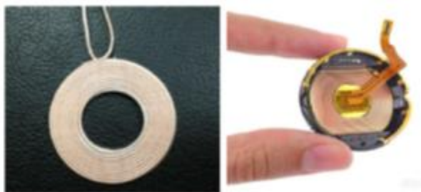
Figure 24: Tony Electronic is Apple's major supplier of wireless charging coils for Apple Watch
