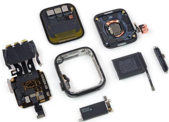
图 31: Apple Watch Series 5 拆分总览
