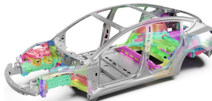
Model 3 body structure, 171 pieces of metal highlighted
