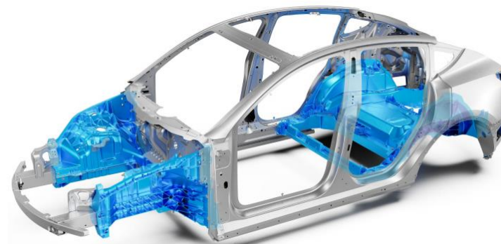
Austin-made Model Y body structure, 2 pieces of metal highlighted, >1600 fewer welds
