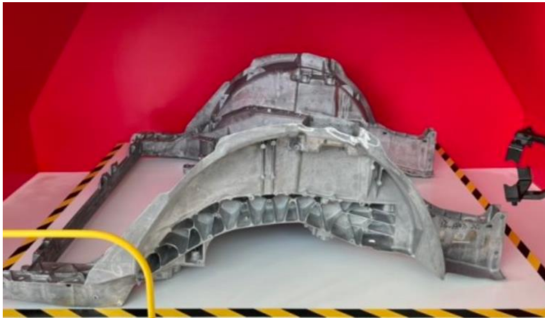
图：Giga Press高速冲压精确度可达到0.01mm
