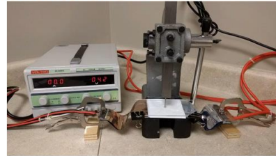
Metallized current collector does not allow current to flow between layers V = 4.0 V, I = 0 A
