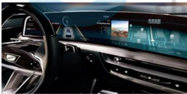
凯迪拉克LYRIQ33英寸Mini LED背光屏
