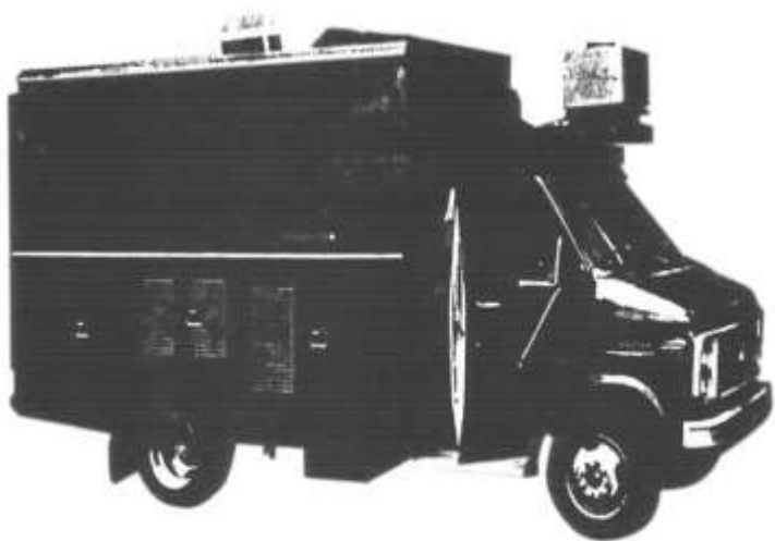
Figure 3: NAVLAB, the CMU autonomous navigation test vehicle.
