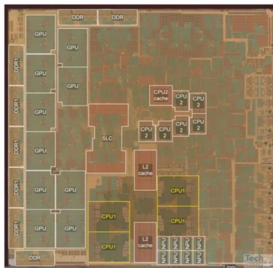
Figure 1 – Apple M4 Die Photograph with Annotated 3-2 and 2-1 finFLEX libraries
