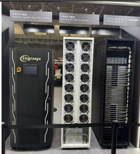
Figure 2: Hon Hai GB200 NVL72 rack at HHTD 2024
