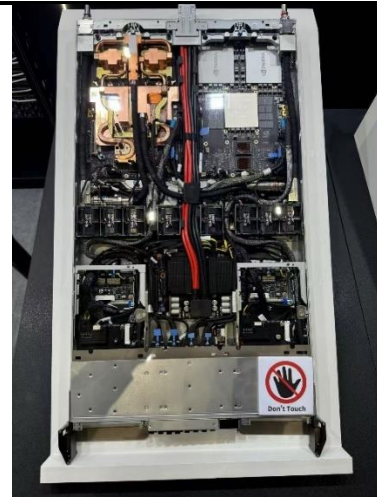
Figure 3: GB200 compute tray at HHTD 2024
