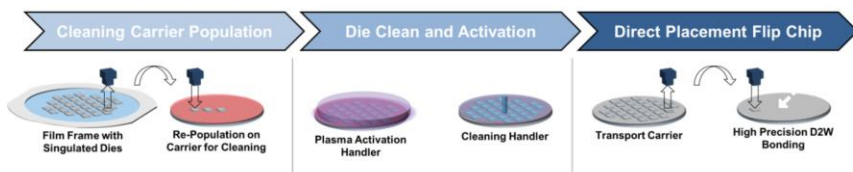
图：Direct Placement D2W bonding 工艺
