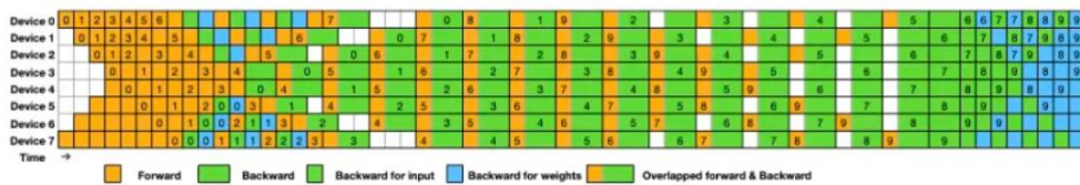
Figure 5 | Example DualPipe scheduling for 8 PP ranks and 20 micro-batches in two directions. The micro-batches in the reverse direction are symmetric to those in the forward direction, so we omit their batch ID for illustration simplicity. Two cells enclosed by a shared black border have mutually overlapped computation and communication.
