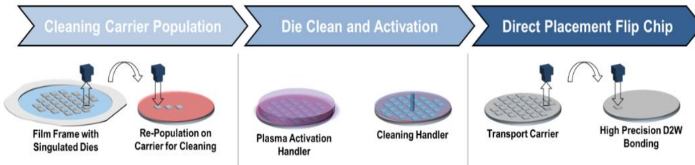
Co-D2W: Collective Die-to-Wafer Bonding
