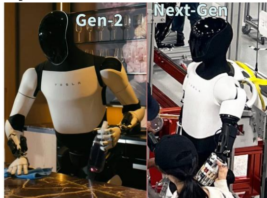
图：Optimus Gen3电机预计整体迁移至前臂
