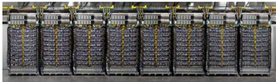
9216 Ironwood Chips Sharing Memory Using OCS
