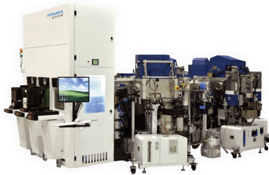
图 11: 北方华创 eVictor 12 Inch PVD System
