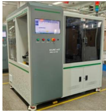
HBQ-Z215B 盲堵盲棒插入机 (长宽高: 1.5m*1.3m*1.8m)
